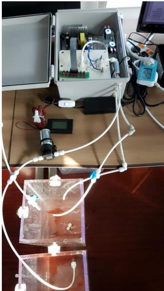
Figure 3: CDI device for desalination performance test
