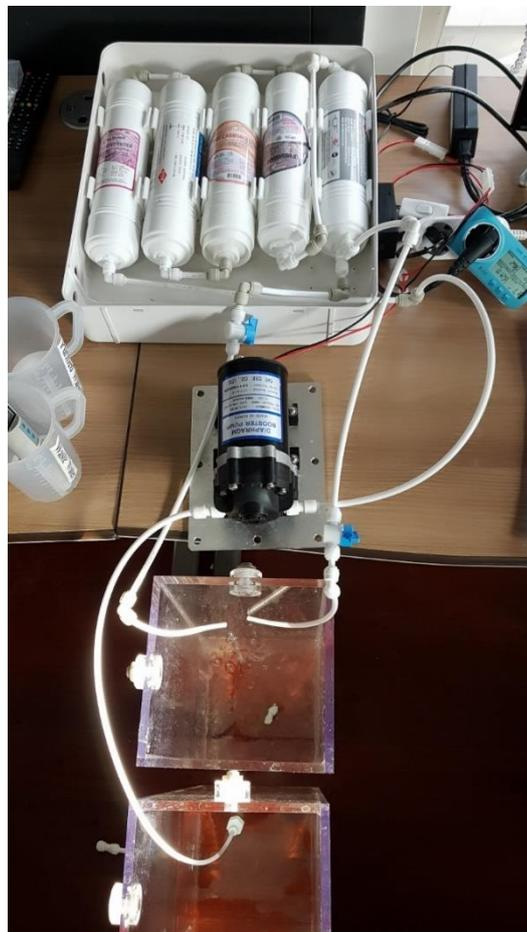
Figure 7: RO device for desalination performance test
